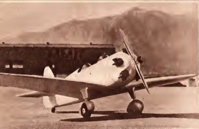
Above is a plastic plane of impregnated spruce plywood and phenol plastic. At the right, Harry Atwood inspects the model of a plastic plane now under construction, which is designed for stratosphere flights. The present war in Europe has spurred interest in the future of plastic planes.
